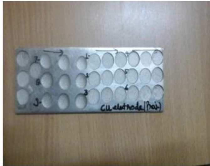
Figure 2.1: Work piece of Inconel 718 after machining with Cu electrode
